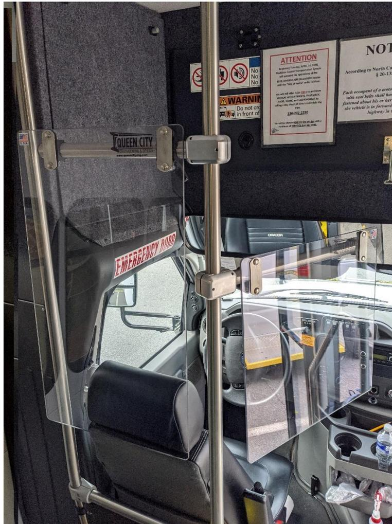
Our shielding systems far surpass others in the market in terms of quality and performance. Made only from American made materials including 1/4" thick polycarbonate, food grade stainless steel, and aircraft grade aluminum, our systems are built to last.
